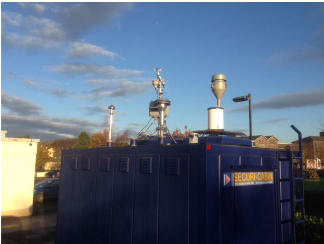
Mobile Air Monitoring Laboratory for measuring gases and properties of particles
