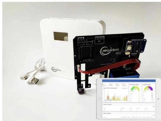
Identical to the PRO kit but all components pre-soldered, the MCU pre-flashed and can be assembled in five minutes. We do also test all components before shipping to ensure you get an accurate and reliable device.
