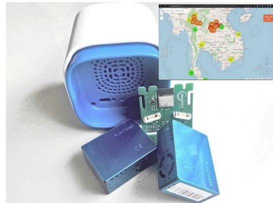
Outdoor air quality monitor with dual PM modules. Measures PM1, PM2.5, PM10, Temperature and Humidity. Comes with pre-assembled PCB and can be built without soldering within minutes.
